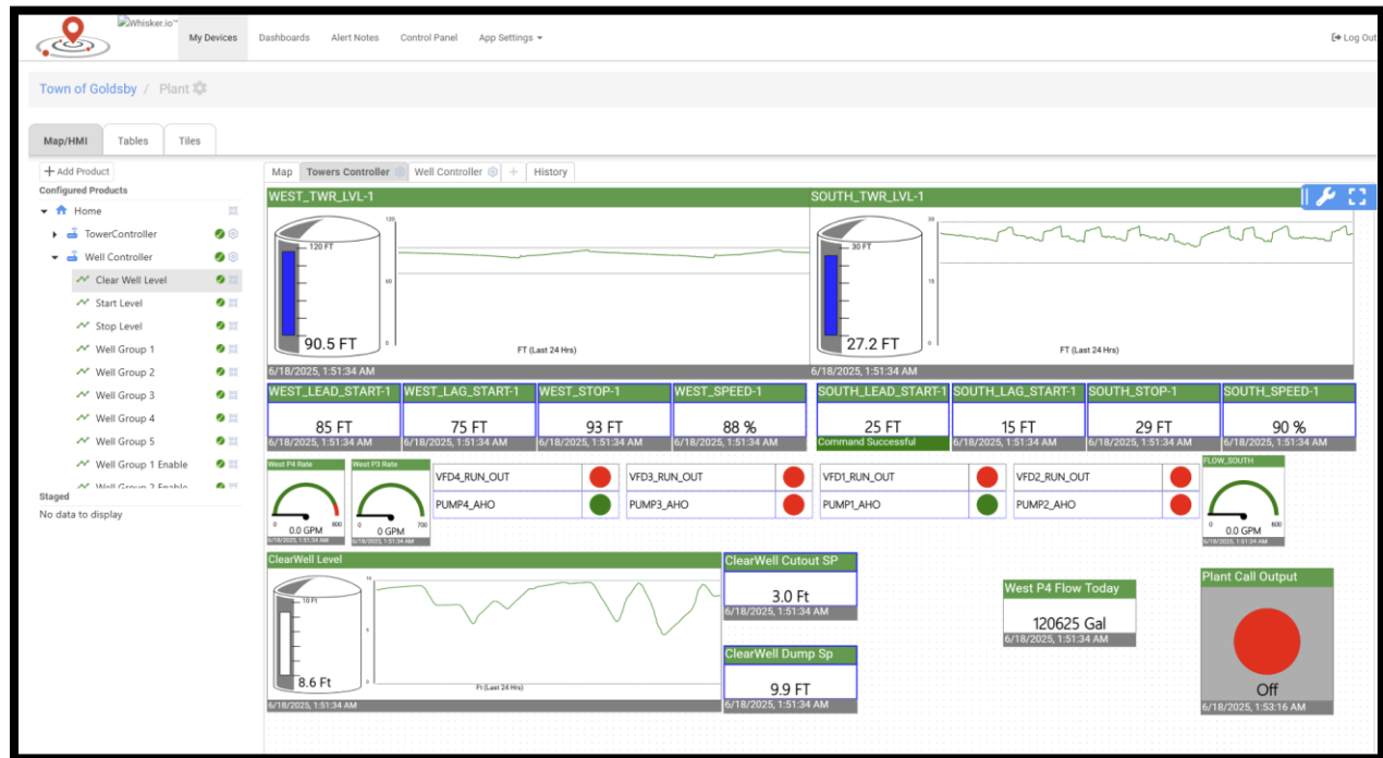
Figure 1: Typical HMI - appearance will vary customer to customer (shared with permission)
